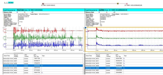
Gambar 4. TWS Reclose Sunyaragi-Arjawinangun I (17 November 2023)
